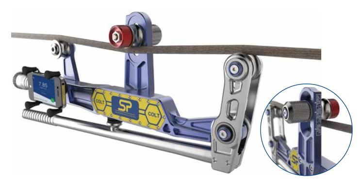
The Straightpoint COLT is a lightweight tensionmeter for fast and accurate measurement of wire rope tensions up to 11,000lbf/5000 kgf and up to 1"/25mm diameter.
